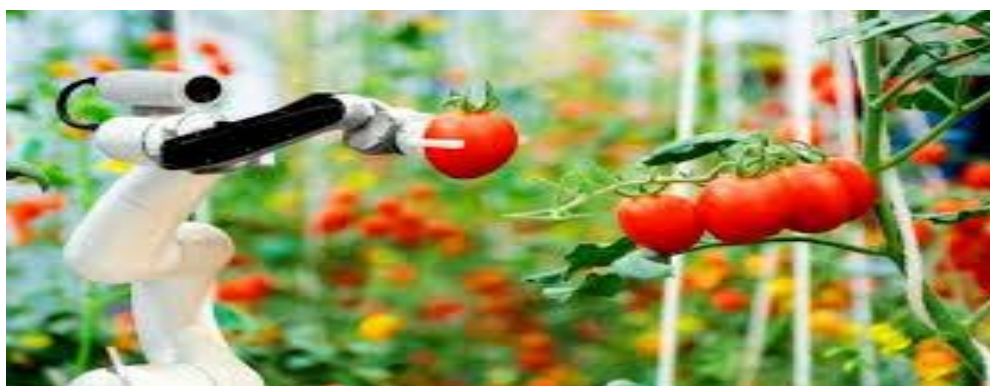
Figure 2, Tomato harvesting using robot Gadha Sreekumar (2023)
